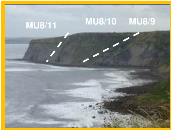
MU8/9 and MU8/11 are Partly Active sea cliffs. MU8/10 is a debris slide deposit classified as Partly Active.
